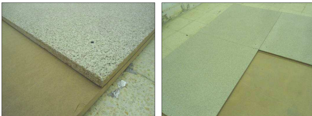
Images 3 and 4 Installation of the test specimen into de reverberant room
